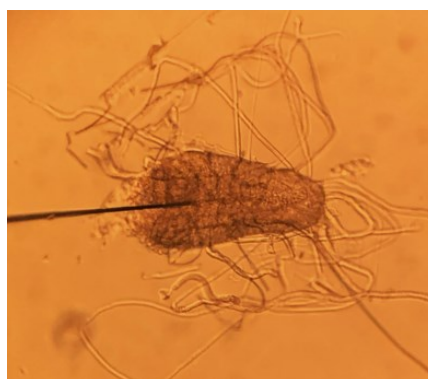
Carbon fiber microelectrode placement in fruit fly larva ventral nerve cord to measure serotonin with fast-scan cyclic voltammetry (FSCV)
